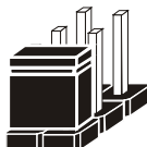
Jumper Block 1-2 pin close(enabled) Looks like this
