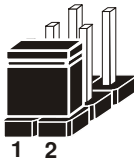
Jumper Block 1-2 pin close(enabled) Looks like this
