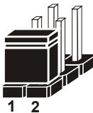
Jumper Block 1-2 pin close(enabled) Looks like this
