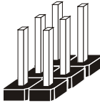
Jumper Block looks like this
