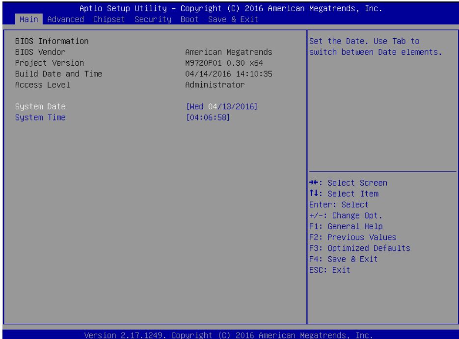
BIOS Setup Program Initialization Screen
