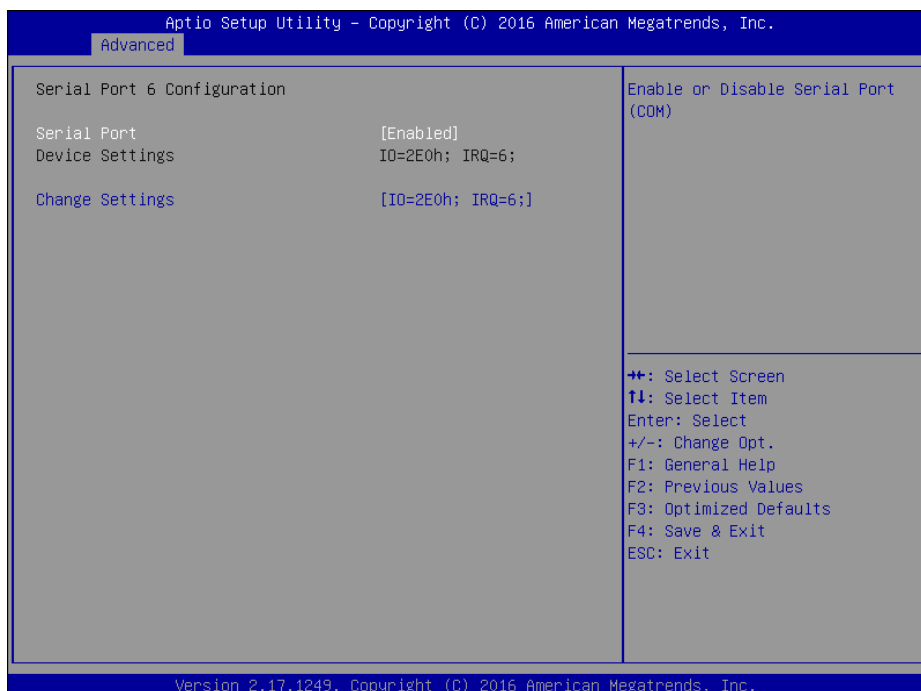
Serial Port 6 Configuration Screen
