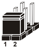
Jumper Block 1-2 pin close(enabled) Looks like this
