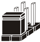
Jumper Block 1-2 pin close(enabled) Looks like this
