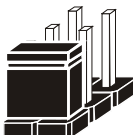
Jumper Block 1-2 pin close(enabled) Looks like this
