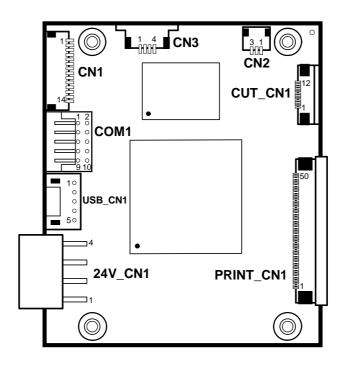
Figure 3-2. MB-1030 Printer Board Component Locations
