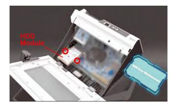
Step 3. Take out the HDD module to complete.
