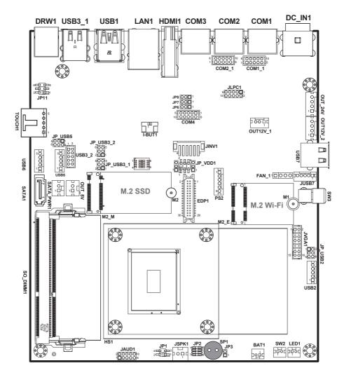
Figure 3-1. Main Board Component Location (Top View)
