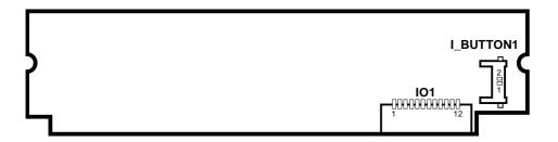
Figure 3-5. MB-3012 MSR Board Component Locations
