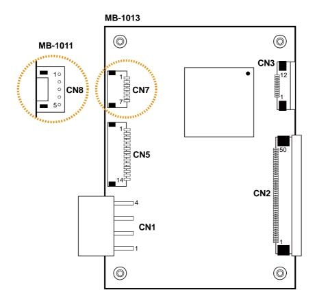
Figure 3-3. MB-1011 & MB-1013 Printer Board Component Locations
