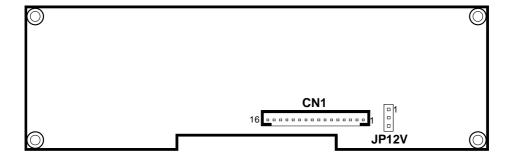
Figure 3-4. MB-4103 & LD720 VFD Board Component Locations
