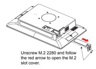
Step 2: Slide a new M.2 2280 into the M2. slot and fasten up the screw to secure the cover and complete.
