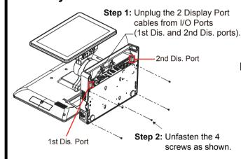
Step 3: Move the PCB box outwards slightly as shown (red arrow) and lay the PCB box down on a flat surface.
