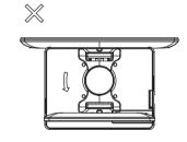
Warning: If you force to turn not in the direction you previously turned, the internal structure of the POS system could be damaged.
