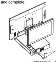
Slide a new M.2 2280 into the M2. slot and fasten up the screw to secure the cover.
