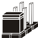
Jumper Block 1-2 pin close(enabled) Looks like this
